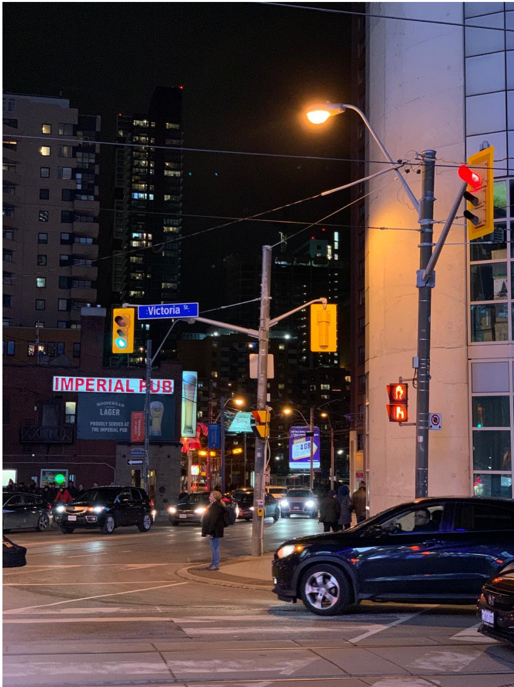
Figure 7: Signal, pedestrian signal, crosswalk, pedestrian, and (in background) pedestrian crossover. Dundas St at Victoria St, looking east.
